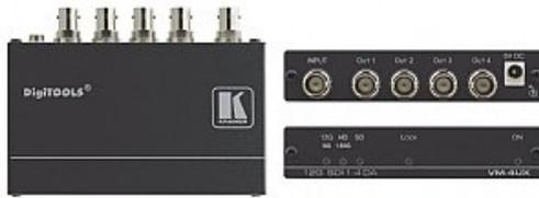
The VM-4UX is a compact and high performance 1:4 4K distributor for standard broadcast-grade SDI signals of up to 12G transmitted data rate. It auto-adapts to the data rate of one SDI input signal, equalizes and re-clocks the signal to improve transmitted signal reach, and distributes the signal to four identical SDI outputs
